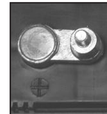
POSITIVE POST HAS LARGER DIAMETER
