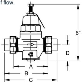
NOTE: If a solder union is to be used, sweat the union tailpiece and nut onto the pipe prior to installing the PRC assembly, otherwise the heat could damage the assembly components.
