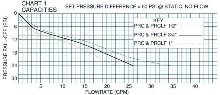
NOTE: Although this chart shows curves at a 50 psi set differential, curves for other settings are similar. The curve shifts slightly to the left for a smaller differential and to the right for a greater differential. The adjustment is as follows: for a 25 psi set differential subtract 15% from the flow rate shown. For a 75 psi set differential add 15 % to the flow rate shown.
