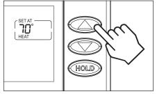
**Press** or to adjust the current setting. In AUTO use MODE to switch between the HEAT and COOL setting.
