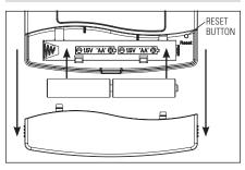
The thermostat can either be AC or battery powered, or both. When wired to be AC powered, the batteries are optional and only provide backup power to the clock.
