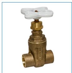
**Specifications UPC** Code 039923309938 Gate Valve Type **Valve Size** 1/2 in Material Lead Free Silicon Bronze **Description** S113-LF 1/2 CXC 300 CWP NRS GATE BRZ Multi-Turn **Turns / Operation** Seat / Seal Material **Bronze Connection Type** S -- Female Solder Cup Valve Gate Stem Design NRS - Non-Rising Stem Valve Multi-Turn Bonnet Design Screw-in Bonnet **Operation Type** Standard Handwheel
