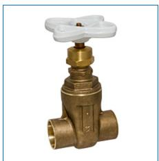
**Specifications UPC** Code 039923309945 Type Gate Valve **Valve Size** 3/4 in Material Lead Free Silicon Bronze **Description** S113-LF 3/4 CXC 300 CWP NRS GATE BRZ Multi-Turn **Turns / Operation** Seat / Seal Material **Bronze Connection Type** S -- Female Solder Cup Valve Gate Stem Design NRS - Non-Rising Stem Valve Multi-Turn Bonnet Design Screw-in Bonnet **Operation Type** Standard Handwheel
