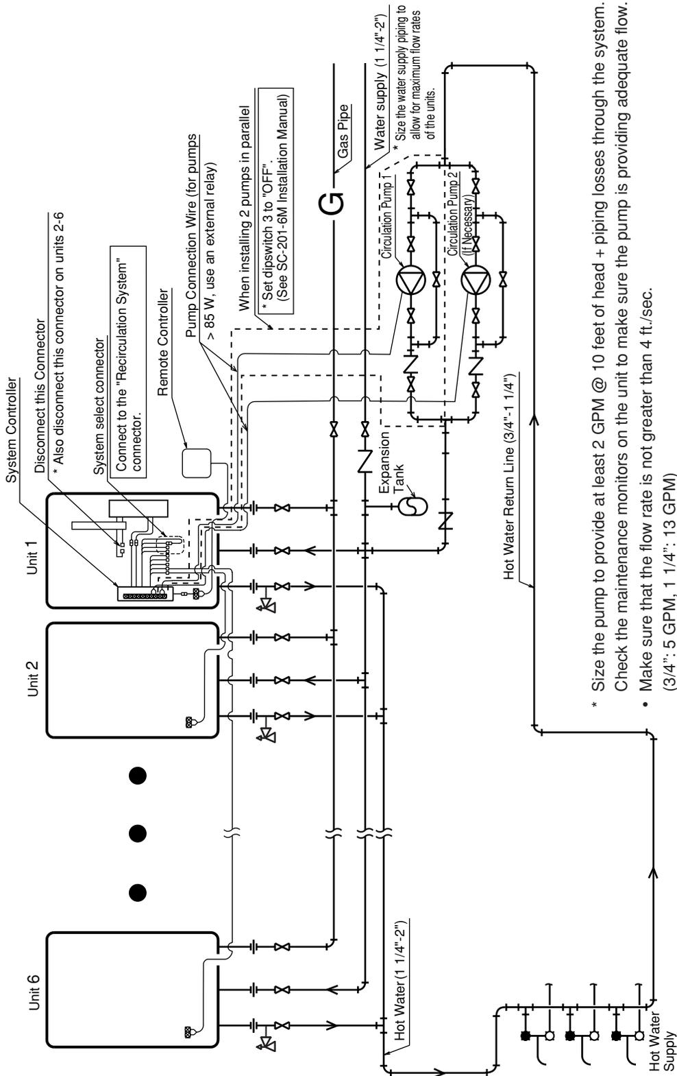
\* Size the pump to provide at least 2 GPM @ 10 feet of head + piping losses through the system.
