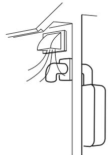
State of California: The water heater must be braced, anchored or strapped to avoid moving during an earthquake. Contact local utilities for code requirements in your area or call: 1-866-766-7489 and request instructions.
