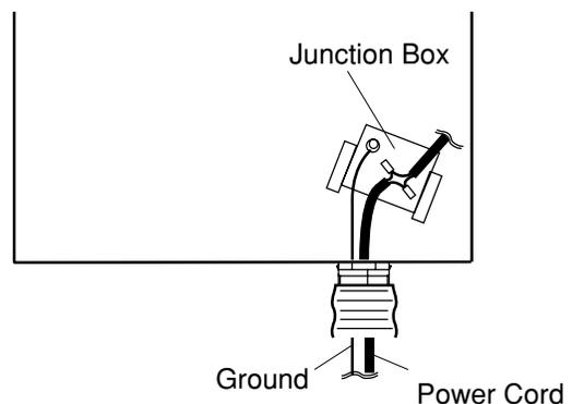
1. Unscrew the junction box and slide it out of the unit.
