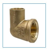
**Specifications UPC** Code 039923333117 **All Type of Item** Fitting **All Special Application** Lead-Free\* **Description** 707-3R-LF 1/2X3/4 CXF 90 ELBOW CAST **Fitting Bend Angle** 90 Deg (1/4 Bend) Elbow **Type Connection Type** C x F (NPT) Weight 0.183 lb Size 1/2 x 3/4 Material Lead-Free Bronze
