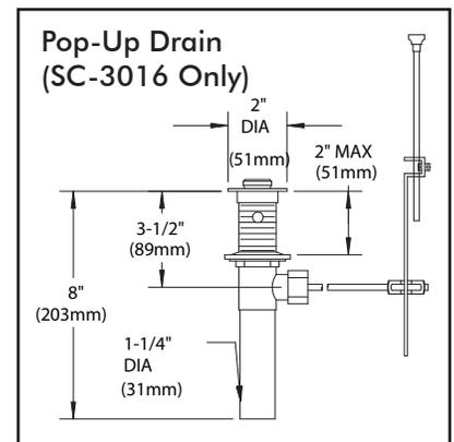
**NOTE:** All dimensions are in inches (millimeters) unless otherwise specified and are subject to change without notice. Lavatory inlets are sized for either coupling or sweat connections. Unless otherwise specified, all inlets are 1/2" NPSM.
