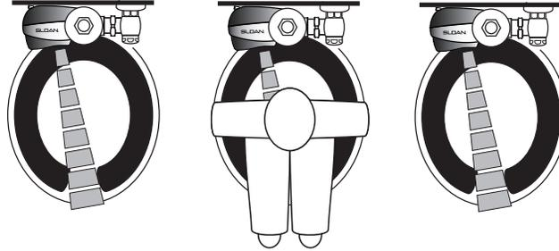
1. A continuous, invisible light beam is emitted from the OPTIMA plus<sup>®</sup> Sensor.
