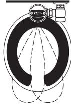
1. A continuous, invisible light beam is emitted from the Sloan ECOS® Dual Flush Sensor.
