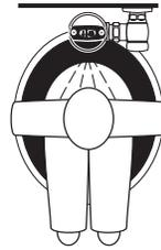
2. As the user enters the beam's effective range, 22 to 42 inches (559 mm to 1067 mm), the beam is reflected into the Scanner Window to activate the Output Circuit. Once activated, the Output Circuit continues in a "hold" mode for as long as the user remains within the effective range of the sensor. If the user stays longer than 65 seconds, a full flush will automatically initiate when the user leaves.
