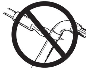
directly to the frozen tubing section. Temperature on tubing shall not exceed 180°F.
