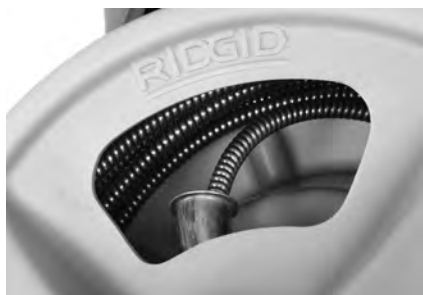
Figure 18 – Coil Cable Into Drum As Shown
