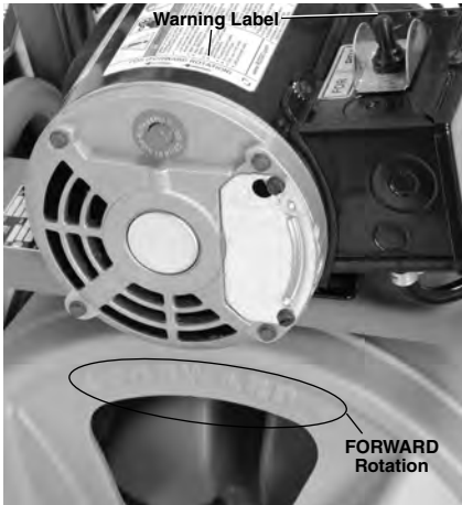
Figure 8 – Proper Drum Rotation (FOR Switch Position)
