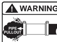
**WARNING** This is a non-restraining product. If pipe pullout can occur proper anchoring of the pipe joint is required. Failure to anchor pipe could result in the escape of line content and may cause property damage, serious injury or death.
