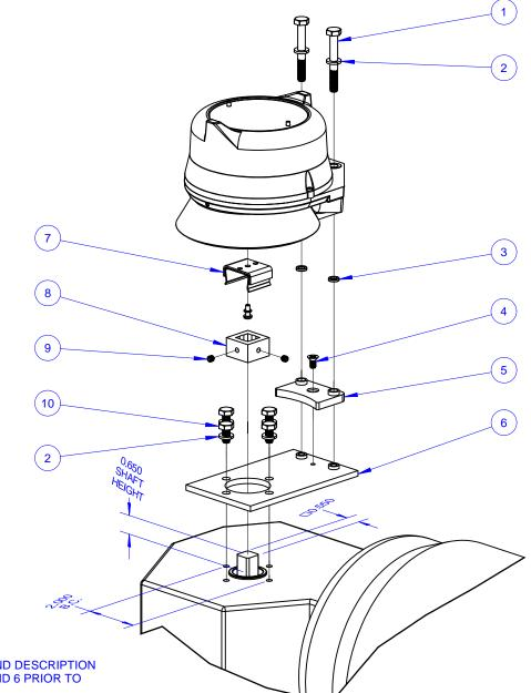
NOTE: 1) SEE BOM FOR PART # AND DESCRIPTION 2) ASSEMBLE ITEMS 4, 5 AND 6 PRIOR TO PACKAGING KIT 3) ASSEMBLE ITEMS 8 AND 9 PRIOR TO PACKAGING KIT
