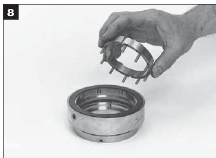
Remove the stationary drive with the springs. Remove the static O-ring from inside the hub gland. Remove the springs from the stationary drive.
