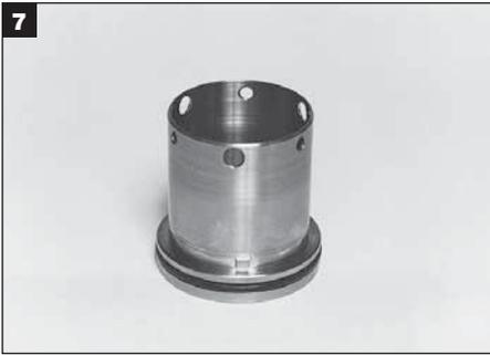
Lubricate the sleeve I.D. O-ring with the silicone grease provided and install it in the sleeve I.D. groove. Lubricate the rotary O-ring and install it in the sleeve O.D. groove.
