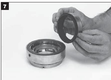
Remove the stationary and the adapter together. Separate them and remove the dynamic O-ring.
