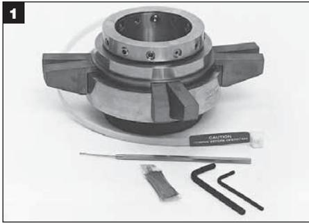
You will need the hex keys provided with the seal, and an O-ring extractor or paper clip to disassemble the seal.
