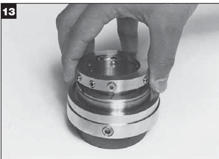
Turn the assembly over and place with the lock ring side of the sleeve up, on a flat surface. Place the lock ring over the sleeve, lining up the flat head socket screws with the smaller holes and the cup point set screws with the larger holes. Press down on the lock ring and tighten the flat head socket screws and the cup point set screws. Check to ensure that the sleeve is not deformed while tightening the set screws. Make sure the screws do not protrude into the sleeve I.D. bore.
