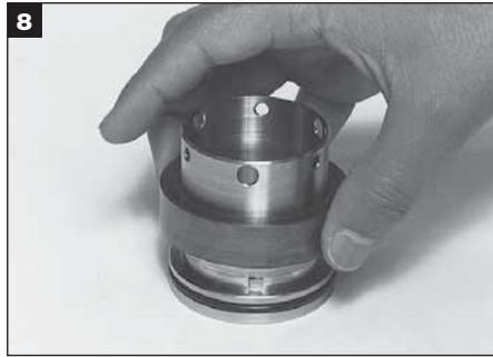
Slide the rotary onto the sleeve, aligning the drive tabs with the rotary slots. Slide the rotary over the O-ring until the rotary bottoms out. Check to make sure the drive tabs are properly engaged.
