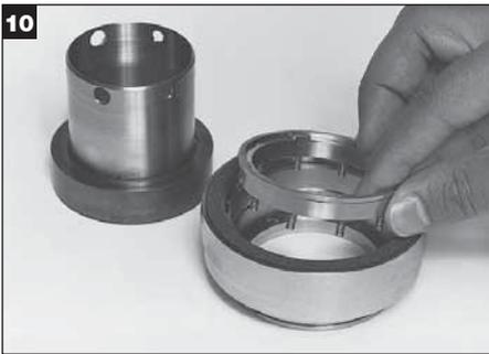
Place the hub gland assembly with the gasket side up, on a flat surface. Align the slots in the stationary drive with the tabs in the hub gland. Slide the stationary drive in until the springs touch the hub gland. Place the back-up washer in the hub gland. It will rest on the stationary drive until the seal is compressed.
