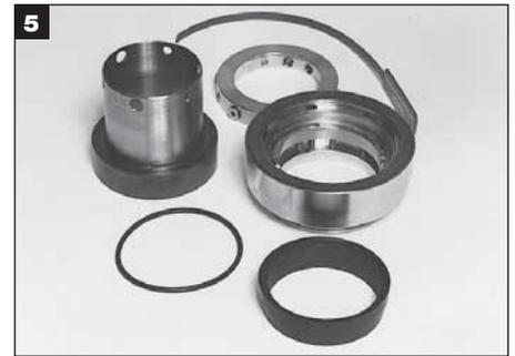
Lift out the stationary and remove the dynamic O-ring.
