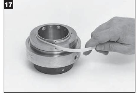
Press down on the hub gland and push the centering strap through the slot in the hub gland. Push the strap in until it completely surrounds the seal sleeve. It will pilot between the hub gland, seal sleeve and lock ring.
