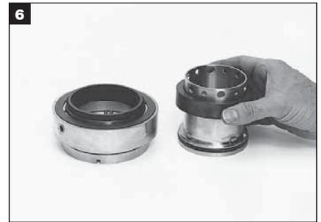
Remove the rotary, rotary O-ring and shaft O-ring from the sleeve.
