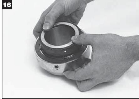
Slide the sleeve, with the rotary installed, downwards into the hub gland. Pick up the hub gland and sleeve and continue to push them together until the faces contact each other.
