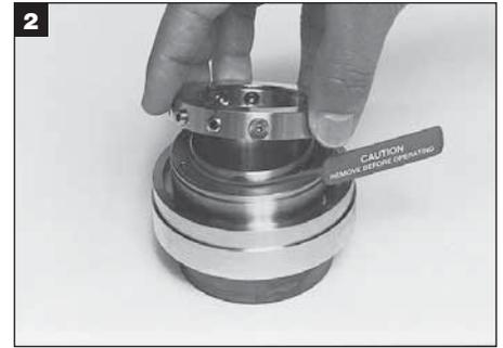
Place the seal, lock ring side up, on a flat surface. Back out all the screws from the sleeve. Remove the lock ring. Remove the centering strap.
