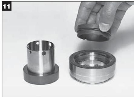
Lubricate the dynamic O-ring for the stationary. Slide the O-ring onto the stationary. Slide the stationary into the hub gland until it engages the stationary drive. Be sure to line-up the drive tabs with the stationary slots.
