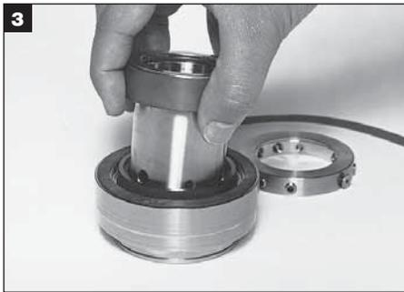
While holding the sleeve and gland together, turn the seal assembly over and lift out the rotary and the sleeve, separating the stationary face from the rotary face with your fingers. Turn the faces in opposite directions if it becomes difficult to separate them.
