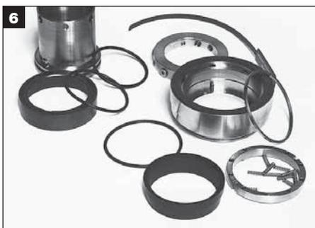
Remove the back-up washer and stationary drive with the springs. Remove the springs from the stationary drive. Remove the rotary, rotary O-ring and shaft O-ring from the sleeve.
