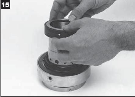
Wipe the stationary and rotary faces clean with a lint free cloth. Place the hub gland, with the stationary installed, stationary side up on a flat surface. Place the stuffing box face gasket in the hub gland.
