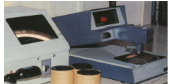
Specialized film reader and digital densitometer are used in interpreting radiographic film.
