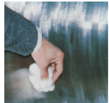
A "Cotton Test" checks the smoothness of the interior surface of pulp mill head box piping.
