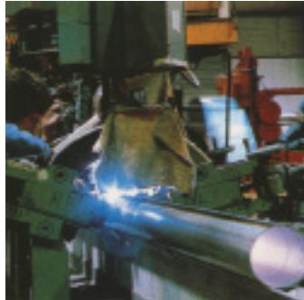
Automatic straight-seam welding from both sides using the gas tungsten arc process produces pipe and tubing in sizes up to 24 inch diameter in continuous lengths up to 20 feet. Sizes up to 60 inch diameter are available using other equally refined welding techniques.
