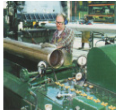
Hydrotesting verifies pressure capabilities of pipe and tubing.
