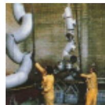
Pickling and passivation enhances the appearance, and in certain cases, the corrosion resistance of Alaskan stainless steel pipe and fittings.
