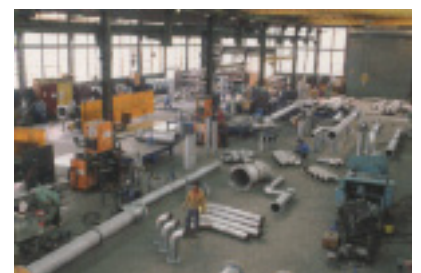
Prefabricated piping systems, produced by our Fabrication Division, result in reduced field welds and installation cost.
