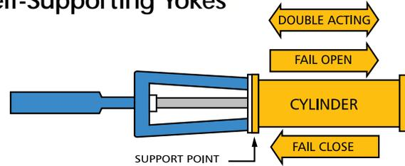
Properly support the cylinder actuator at the yoke operator mount plate, when the valve is mounted in a position other than stem-vertical; the support can be a pedestal from the bottom or support from the top. Spring return cylinders may require additional support at the top of cylinder due to length and weight. Cylinders in harsh vibration service may require additional support or damping at the top of the cylinder.
