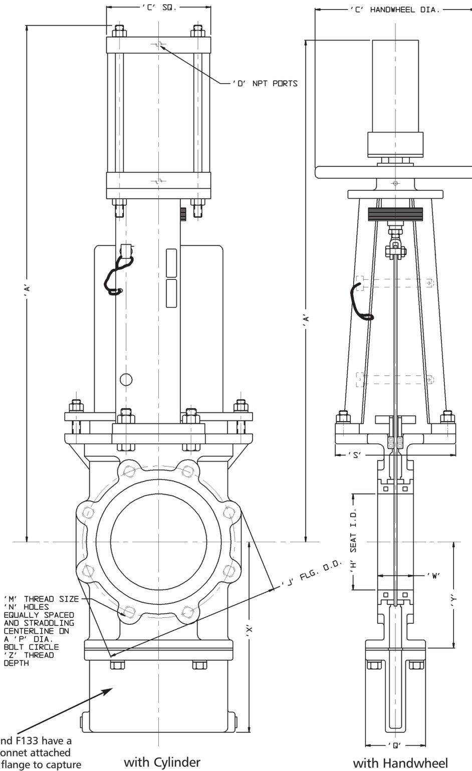
Figures C133 and F133 have a containment bonnet attached to the bottom flange to capture any discharge during cycling.
