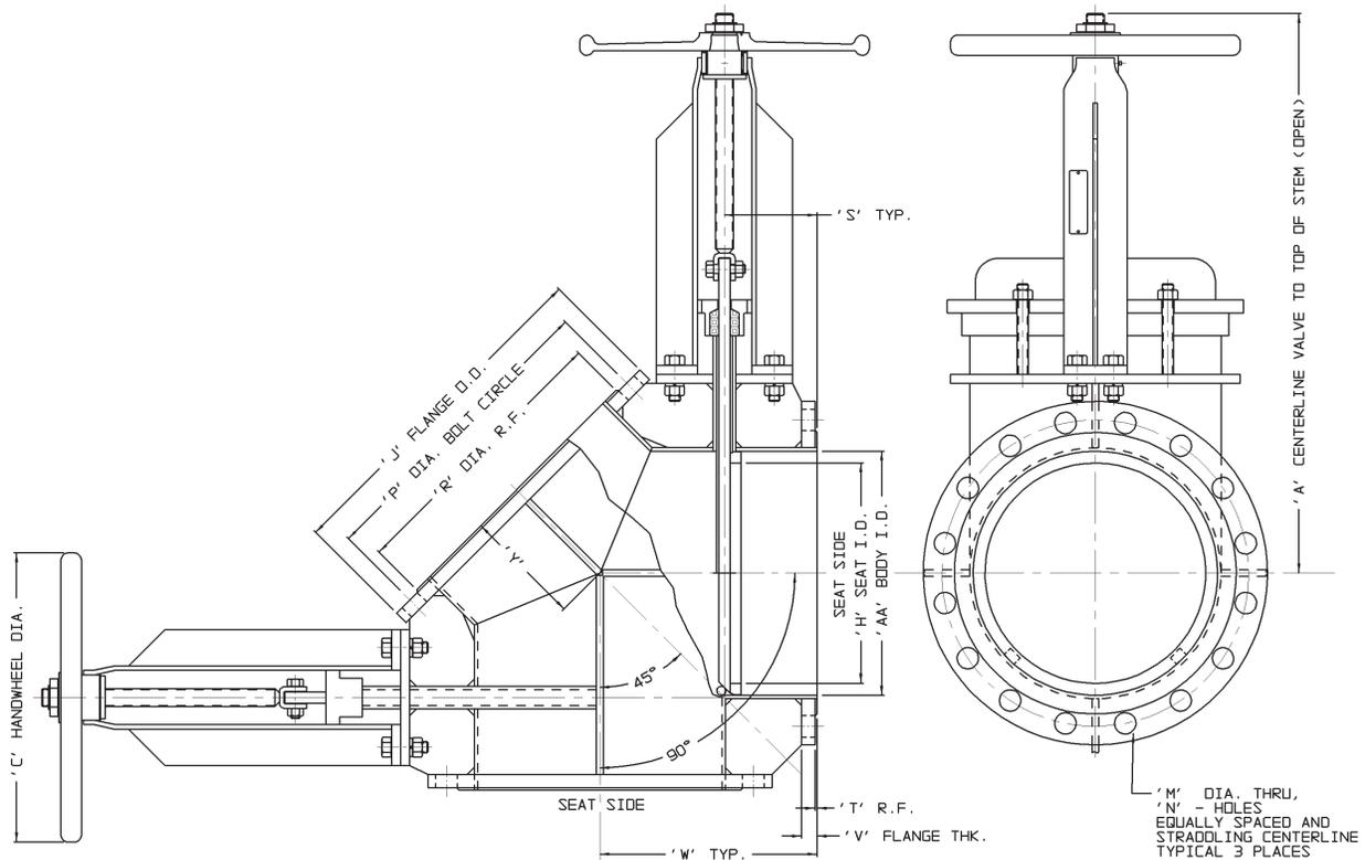
Actuator orientation and the angles between the legs can be varied to suit the application. The typical Figure F44 has one inlet with two, three or more outlets. However, the figure F44 design platform is extremely flexible; therefore designs including single or multiple inlets with single or multiple outlets can easily be manufactured.
