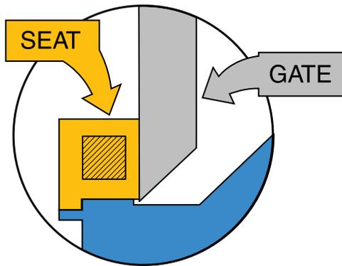
**Polyurethane (RP)** replaceable seats are designated "RP". Polyurethane is excellent in abrasive applications. A heavy steel internal reinforcing ring insures that the Polyurethane holds its shape and remains in place. Gaskets are not used with this seat. Maximum temperature is 180°F (82°C).
