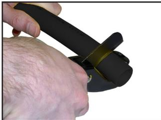
**4** Chamfer end of pipe using [Continental's ID chamfering tool with ID gauge](#).
