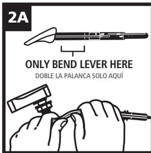
**2A** For side or angle-mount: slowly bend new lever arm to match shape of old lever arm. (See picture where to bend lever). DO NOT bend arm quickly or back and forth repeatedly.
