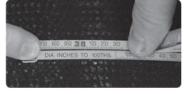
...Trumbull's 10 foot tapes can measure the outside diameter of 36" ductile pipe (38.30" O.D.)
