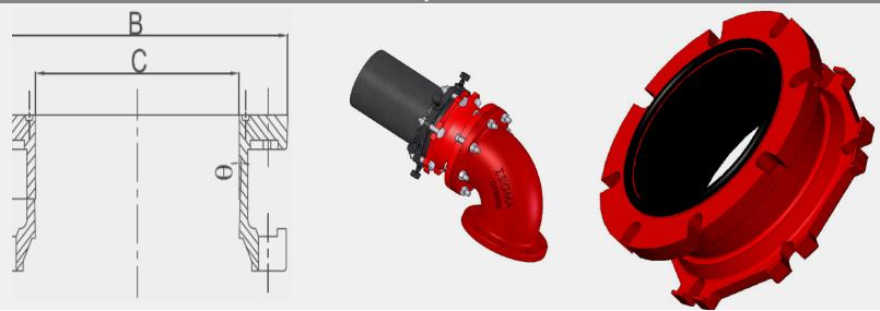
SIGMA Corporation's SIGMAFLANGE Model SFA is designed to connect plain-end ductile iron or PVC pressure pipe to a flanged fitting, pipe, valve and other flanged appurtenances. An oversized ductile iron mechanical joint x flanged sleeve provides proper sealing of the adjacent flange outlet using an O-ring gasket while accommodating necessary pipe end restraint to the mechanical outlet using SIGMA ONE-LOK<sup>™</sup> SLDE for ductile iron or SLCE for PVC pipe wedge-action restraining gland.
