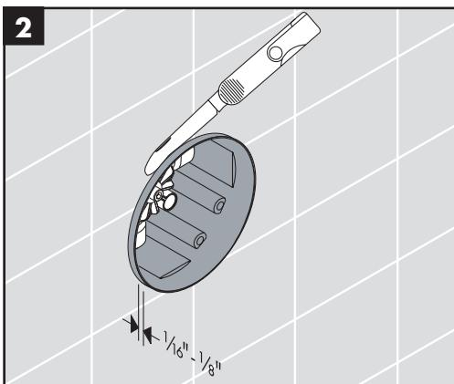
Cut the plaster shield so that it extends  $\frac{1}{16}$ " -  $\frac{1}{8}$ " from the finished wall surface.
