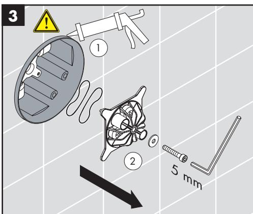
⚠ Seal the wall around the plaster shield with waterproof sealant (1).
