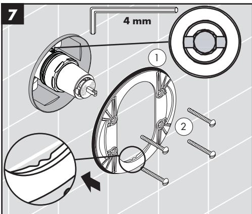
Open the stops using a 4 mm Allen wrench (1).
