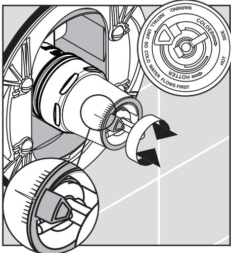
Turn the rotational limit stop, clockwise to make the water cooler, counter-clockwise to make it warmer.
