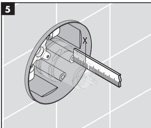
Measure the distance from the front of the plaster shield to one of the screw-in flanges ("X").
