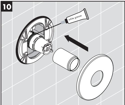
Lubricate the cartridge o-ring using a small amount of white plumber's grease.
