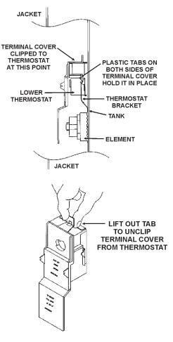
B. **Models with Upper or Lower Thermostat with High Limit:** Lift out the tab as shown below to unclip the terminal cover from the thermostat. The terminal cover can now be removed from the thermostat.
