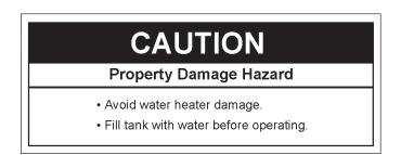
Never use this water heater unless it is completely full of water. To prevent damage to the tank and heating element, the tank must be filled with water. Water must flow from the hot water faucet before turning "ON" electrical supply to the water heater. The manufacturer will not warrant any elements damaged by failure to follow instructions.
