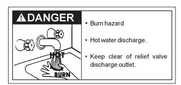
The temperature-pressure relief valve must be manually operated at least once a year.
