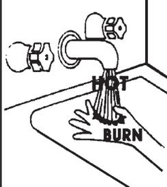
**⚠ DANGER** Water temperature over 125°F (52°C) can cause severe burns instantly resulting in severe injury or death.
