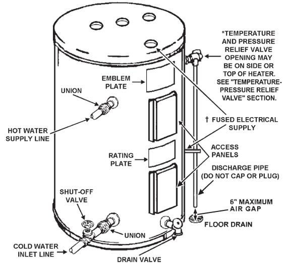
↑ ELECTRICAL CONNECTIONS MAY BE LOCATED ON THE TOP OR SIDE, REFER TO YOUR UNIT. ACTUAL MODEL AND ILLUSTRATION MAY VARY DEPENDENT ON MODEL CAPACITY AND TYPE. SOME MODELS HAVE ALTERNATE INLET, OUTLET AND T&P VALVE LOCATIONS. THESE ALTERNATE LOCATIONS ARE IDENTIFIED BY THE LABELING ON THE UNIT.
