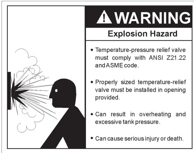
This heater is provided with a properly certified combination temperature - pressure relief valve by the manufacturer.
