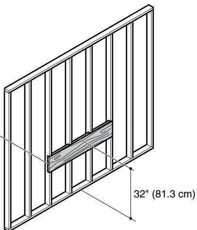
**NOTICE:** To properly secure the vanity, the top of the required 2x6 backing material must be 32" (81.3 cm) from the finished floor.
