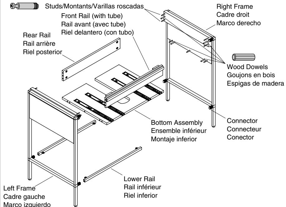
**NOTE:** Slight pressure might be needed to assemble the components.
