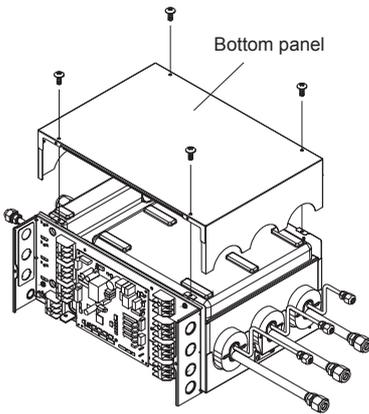
(8) Secure the control box with the screws (4 pieces).
