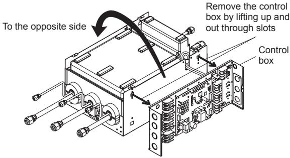
(6) Attach the control box to the main unit as shown in the figure.
