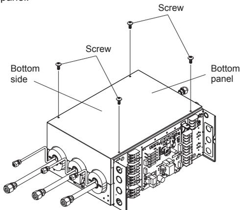
(5) Remove the control box as shown in the figure, and then change the positioning to the opposite side.
