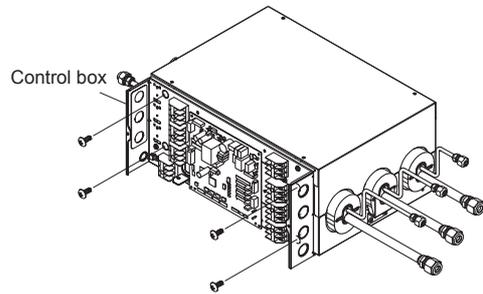
(9) Attach the control box cover and secure it with the screws (2 places).
