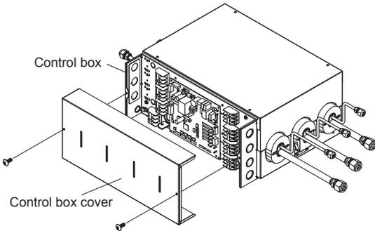
(10) Attach the wiring cover and secure it with the screws (2 places).
