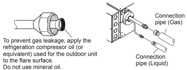
(3) When the flare nut is tightened properly by hand, use a torque wrench to finally tighten it.
