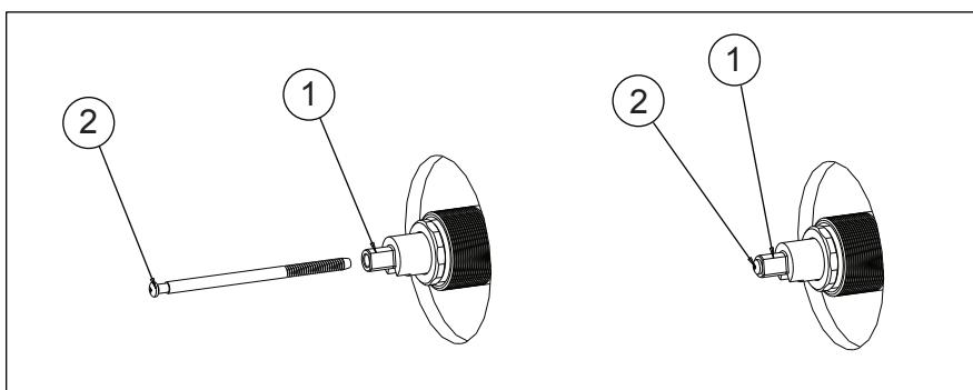
Thread handle screw (2) until it bottoms out in the extender (1).
