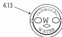
4.13 Cast iron water lid with two hole erie pattern and brass insert threads
