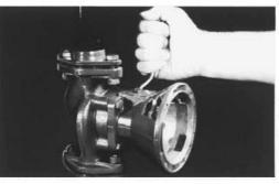
Loosen the four body cap screws. Shift the bearing assembly position slightly to allow for any pressurized water to escape. Remove the four body cap screws.
