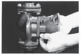
Fit the Bearing Assembly into the Pump Body and tighten Cap Screws evenly. Do not over tighten.
