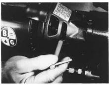
The coupler is loosened by means of backing off the set screw with an Allen Wrench on the pump shaft coupler half. The T-Handle Allen Wrench shown is provided with the B&G Service Kit, but a conventional L-Handle will do the job.
