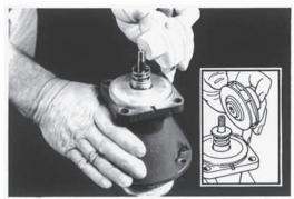
Remove the Impeller Nut and Impeller. Important: Note the following before installing impeller on new bearing assembly. If impeller is metal with flat back as illustrated in insert, the brass metal washer must be used atop the seal spring. If the impeller has a shroud on the back, DO NOT USE THE BRASS WASHER.
