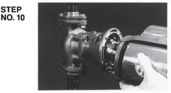
Connect the coupler to the Bearing Assembly Shaft and reposition motor.
