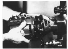
With the cap screws removed, the motor is backed off and if the set screw is backed off the pump shaft sufficiently, the coupler should slide free of the pump shaft. A screwdriver may be used to pry it loose if tight.
