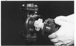
Pull the Bearing Assembly from the Pump Body.
