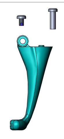
015550-45 (1) Lever Arm Repair Kit w/ Screw and Nut
