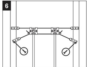
6 Bend bottom bracket as close as possible to LockBlock and secure bottom bracket to stud.
