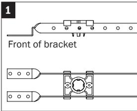
Lay a pair of StrongArm brackets in the upper and lower bracket slots of the male LockBlock.
