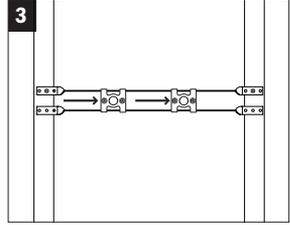
3 With bottom bracket still loose, slide LockBlocks across brackets to desired stub out location.
