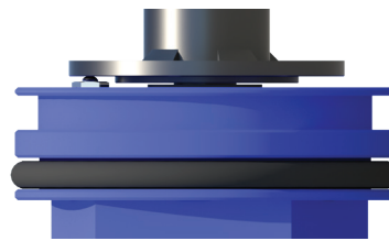
Figure C-5a — Insertion tool making contact with the auto equalization pin.
