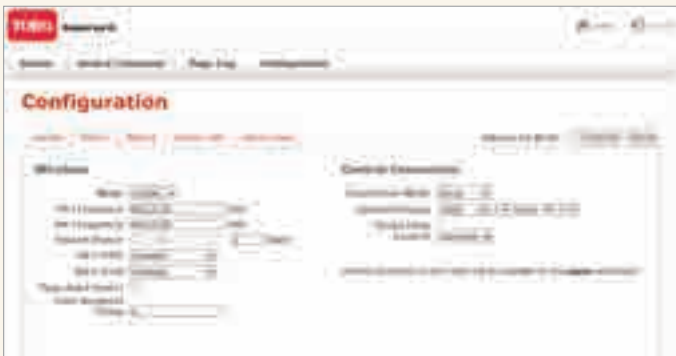
Radio Interface Unit (RIU) Graphical User Interface.
