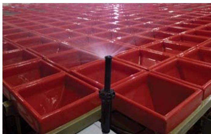
Precision™ Series Spray Nozzles tested higher than competitive water conserving nozzles in multiple independent third party studies for distribution uniformity. The 1"/hr. precipitation rate ensures irrigation runtimes can be achieved even with tight watering windows.
