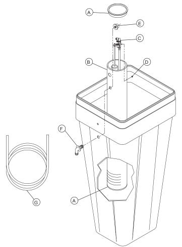
ASSEMBLE THE BRINE TANK: Install a brine well cap (Item A) on the bottom of the brine well (Item B). Remove the brine valve assembly (Item C) from the brine well by removing the nut (Item D). Attach the brine well to the brine tank with the two-piece overflow (Items E & F) using the lower holes in both pieces, as shown. Reinstall the brine valve assembly. Push brine line polytube (Item G) through the upper holes in the brine tank and brine well and press the polytube into the elbow fitting.
