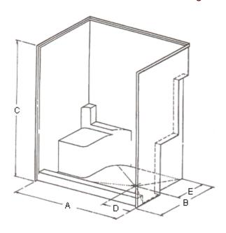
Note: For Flush or Level Use Unit Must Be Recessed Into Floor
