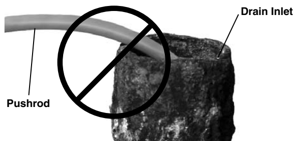
Figure 23 – Avoid Pulling At Sharp Angles
