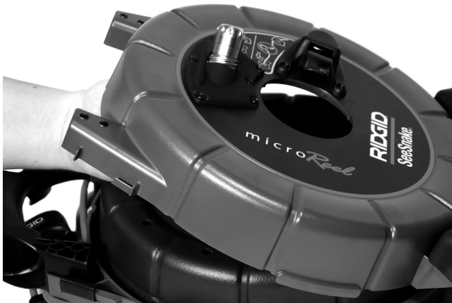
Figure 5 – Open Drum Carefully To Route Cable
