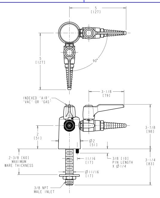
DIMENSIONS ARE IN INCHES AND [MILLIMETERS].
