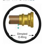
The drip fit O-rings ensure that an unpressed end will drip. This is an added safety feature to ensure unpressed ends are discovered and corrected.
