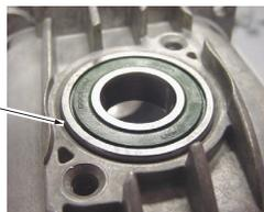
**● LUBRICATION: Type 'L' Grease No. 49-08-4175 (16 oz. tub)**
