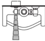
1. A continuous, invisible light beam is emitted from the OPTIMA Sensor.
