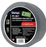
14.0-mil specialty grade cloth duct tape coated with a natural/synthetic rubber adhesive and used to seal, seam and join Class 1 Flex Duct. Excels in usage where tensile strength and adhesion to stainless steel and polyethylene must meet or exceed the strict requirements of UL, flex duct manufacturers, and city and state codes.
