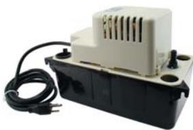
A vertical type pump with stainless steel motor shaft, rust proof, high-impact ABS volute, tank and motor cover, removable 3/8 in. O.D. barbed check valve. Three top inlets provided.
