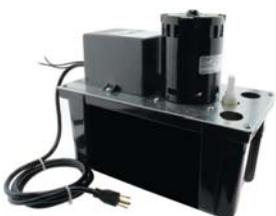
Features a stainless steel motor shaft, ABS tank, and galvanized steel tank cover. Discharge is a 1/4 in. NPT or 3/8 in. O.D. barbed tubing adapter. Two top inlets provided.
