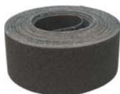
Aluminum oxide high quality 120 grit abrasive cloth for cleaning copper and steel tubing; works wet or dry.
