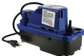
A vertical type pump with stainless steel motor shaft, rust proof, high-impact ABS volute, tank and motor cover, removable 3/8 in. O.D. barbed check valve. Three top inlets provided. Features
