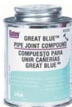
A blue colored non-separating thread sealant compound formulated to seal threaded connections on metal and plastic pipe up to and including two inch diameter. Fibrous texture enhances the sealing properties. Permits easy disassembly without stripping or damaging
