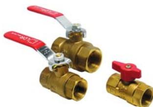
For use with Natural Gas, LP, manufactured and gas-air mixtures. Two-piece brass body and chrome-plated forged brass ball. Heavy-duty valves have a two-piece forged brass body.
