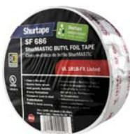
Mastic duct sealer with a paintable printed 2 mil aluminum foil backing and a non-flammable, 100% solid, butyl rubber adhesive. Typical applications are sealing flex duct - both indoor and outdoor. SF 686 also functions well as a permanent, water resistant indoor/outdoor sealer.
