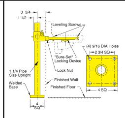
**WELDED BASE** Regularly Furnished. Round steel upright with welded base. Used with floor mounted fixture supports. The base should be securely anchored to the floor construction w/(4) 1/2" bolts. (By others)
