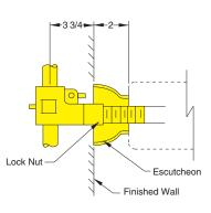
**SUFFIX -E** Threaded Escutcheon. When using lavatories of the flat slab type, the manufacturer requires a 2" dimension from the face of the wall to the rear of the lavatory. The 2" dimension prevents water from accumulating at the wall and causing deterioration. The escutcheon is chrome plated and is available on all concealed arm type supports. Add Suffix -E to figure number required.
