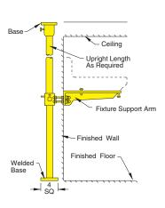
SUFFIX -M11 Floor-to-Ceiling Uprights When required, floor mounted fixture supports can be supplied with floor-to-ceiling uprights for securing to the floor and to the ceiling above. Add Suffix -M11 to figure number required.
