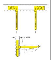
SUFFIX -Z Special Narrow Sleeve and Base for Concealed Arm Support. When a concealed arm lavatory support is to be installed in a narrow wall, a special narrow concealed arm sleeve and base are available for this type of installation. Add Suffix -Z to figure number required.
