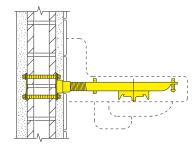
**WALL MOUNTED SUPPORT** - The function of this support is to provide for securing of the fixture to the wall in areas where a floor mounted support cannot be installed. The wall structure must be of sufficient strength to support the entire weight of the fixture.
