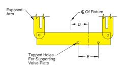
**SUFFIX -KF** Supporting Bar for Fixture Mounted Knee-Action Valve. Can be furnished on any exposed arm, wall or floor mounted sink support. Add Suffix -KF to figure number required.
