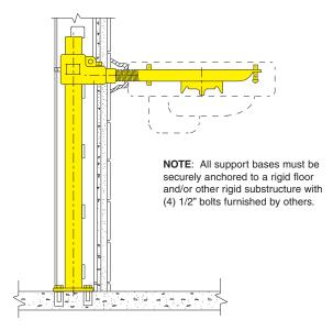
"PRO-SET" FLOOR MOUNTED UPRIGHT SUPPORT - "Pro-Set" is the trade name for the Smith system using uprights welded to base plates. This applies to round or rectangular uprights. The function of the support is to provide the means of mounting an off-the-floor fixture so that the vertical load bearing members are completely concealed inside the wall. This system has no external contact with the finished floor inside the room.
