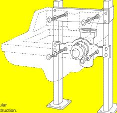
**NOTE:** It is recommended that Suffix -M31, 1 x 3 rectangular uprights (as shown) be used in non-load bearing wall construction.
