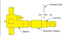
SUFFIX -M24 Extension Adaptor for Concealed Arm Support. When the standard (3 3/4") dimension from the face of the wall to the centerline of support upright, as shown in the illustration, is exceeded, use Suffix -M24 extension adaptor. The face of the extension adaptor should be set 1/2" in back of finished wall so the standard concealed arm and locking arrangement can be used for the lavatory regardless of the wall thickness. Add Suffix -M24 to Fig. No. required.
