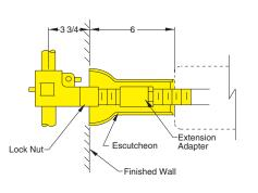
**SUFFIX -E6** <u>6" Long Threaded Escutcheon.</u> When lavatories of the flat slab type are to be set away from the wall beyond the normal 2" setting, a 6" long escutcheon is provided with the same threaded arrangement as the regular 2" escutcheon. This escutcheon is chrome plated and is available on all concealed arm type supports. Add Suffix -E6 to figure number required.
