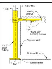
SUFFIX -M31 Rectangular Steel Uprights with Welded Bases. For use with metal stud and sheet rock wall construction. The rectangular shape upright offers greater structural strength and does not rely on the wall construction for support of the fixture. The rectangular upright keeps deflection to a minimum. For use with all floor mounted fixture supports. Add Suffix -M31 to figure number required.
