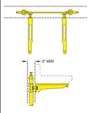
SUFFIX -Z Special Narrow Sleeve and Base for Exposed Arm Support. When an exposed arm lavatory or sink support is to be installed in a narrow wall, a special narrow sleeve and base are available for this type of installation. Add Suffix -Z to figure number required.
