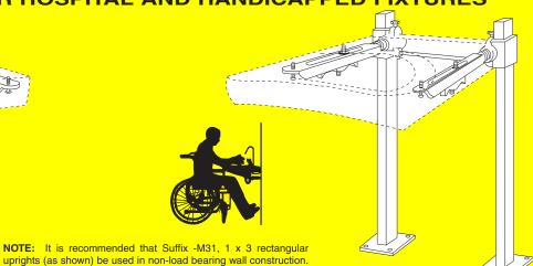
Surgeon's Lavatory - With pedal operated mixing valve for use in patient care areas. Specify Fig. 0700 (-E-KW-M31).
