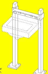
NOTE: It is recommended that Suffix -M31, 1 x 3 rectangular uprights (as shown) be used in non-load bearing wall construction.
