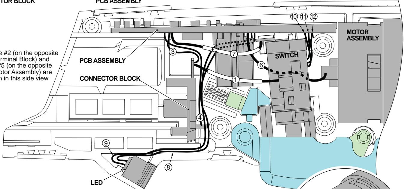
**AS AN AID TO REASSEMBLY, TAKE NOTICE OF WIRE ROUTING AND POSITION IN WIRE GUIDES AND TRAPS WHILE DISMANTLING TOOL.**
