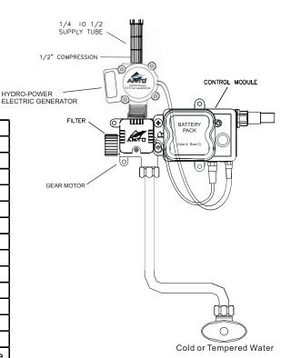
Shown using plug-in hydro-generator.
