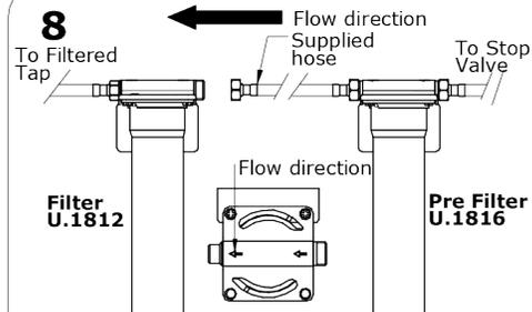
Tighten the hoses from the stop valve to the housings following the flow of the water shown on the cap. When installing the Pre-filter the system flows from the stop valve to the Pre-filter and on to the filter housing and then up to the filter tap.
