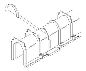
A bottom outlet is attached to the bottom side of the trench drain as shown above. If external ribbing conflicts with the location of the outlet, simply remove the ribbing with a reciprocating saw. A hole saw can be used to cut the appropriate size hole through the bottom of the trench. Attach the bottom outlet with the hardware provided.
