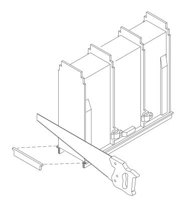
This can be easily accomplished with the use of a hand saw or power reciprocating saw. Use the bottom ledge of the end cap as a guide.
