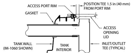
Note: Illinois requires a 6-inch-diameter (150 mm) drop for inlet tee.
