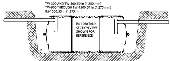
8. Install lids and risers (see Installing Risers section) as necessary.
