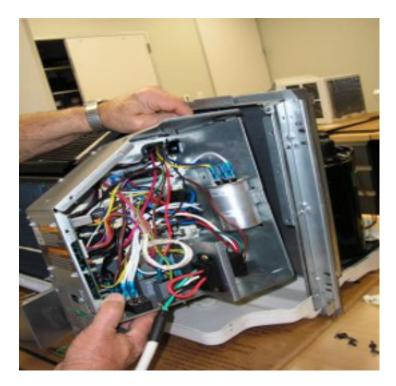
Figure 417 (Removal of Control Compartment)
