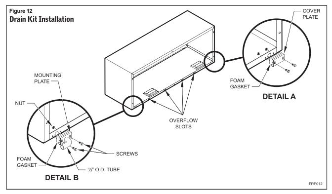
NOTE: The large flange on the mounting plate is positioned at the bottom of the sleeve facing toward the sleeve. The drain tube must be rotated to a horizontal position to allow for the wall sleeve to be installed into the wall. Once the wall sleeve is installed, return the drain tube to a downward angle.
