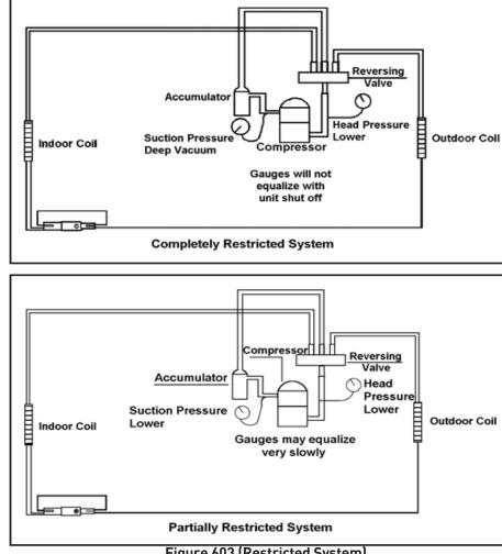
The following conditions are based primarily on a system in the cooling mode.
