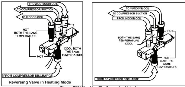
Figure 703 (Checking The Reversing Valve)
