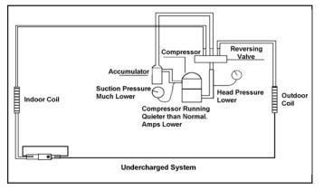
Figure 601 (Undercharged System)
