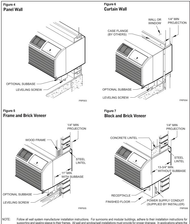
NOTE: Follow all wall system manufacturer installation instructions. For sunrooms and modular buildings, adhere to their installation instructions for supporting and sealing sleeve to their frames. All wall and window/wall installations must provide for proper drainage. In applications where the drain holes on the PTAC wall sleeve are not exposed beyond the wall an internal drain system is recommended. It is the installer's responsibility to ensure there is adequate drainage for the PTAC unit.
