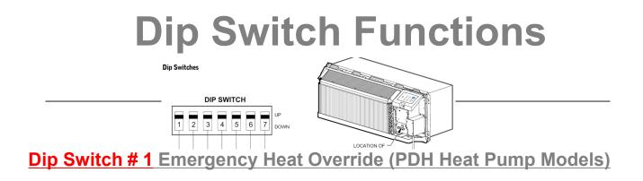
Enables electric heat operation only, in the event of compressor failure
