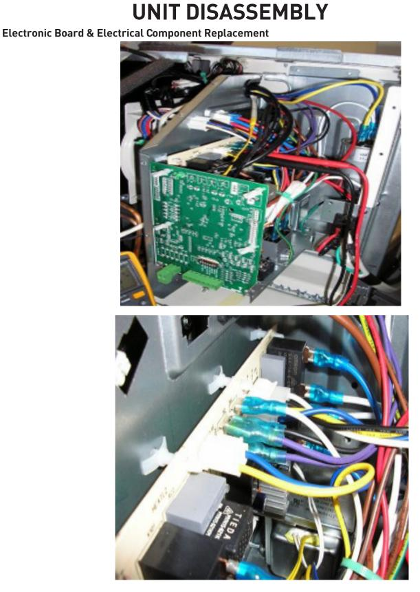
Figure 418 (Main Board & Relay Board)
