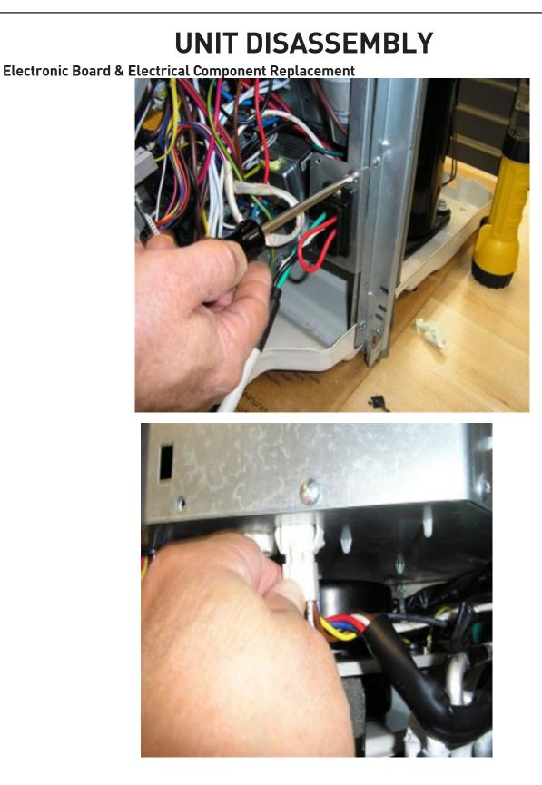
Figure 416 (Power Cord, Indoor Motor, and Heater Connections)
