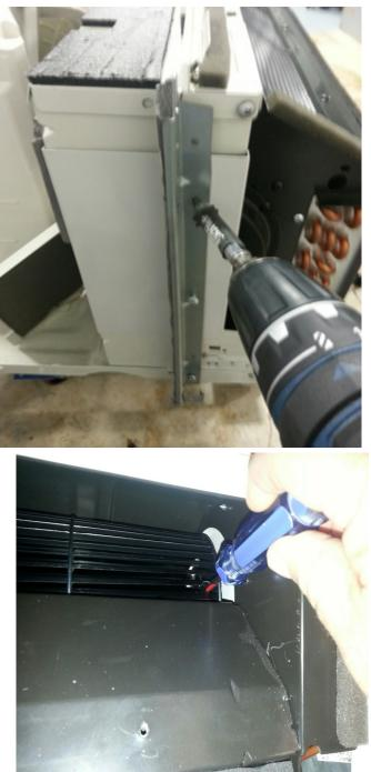
FIGURE 402 (Removal of Indoor Fan Blower Assembly)
