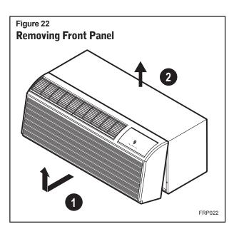
Pull out at the bottom to release it from the tabs (1). Then lift up (2).
