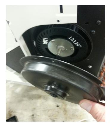
Figure 404 (Left side Bushing & Bushing Housing)
