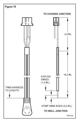
Route the cut ends of harness through the conduit connector assembly and flex conduit sleeve. Be sure to use the supplied conduit bushing to prevent damage to the cord by the conduit.
