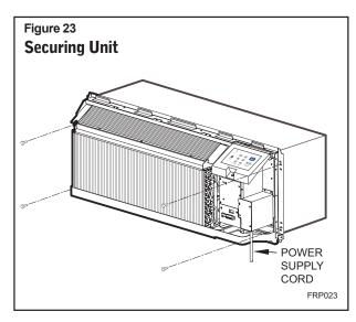
2. Locate the four supplied chassis mounting screws. Insert the screws through the chassis mounting flange holes that are aligned with the speed nuts in the wall sleeve. Tighten all four screws (two per side).
