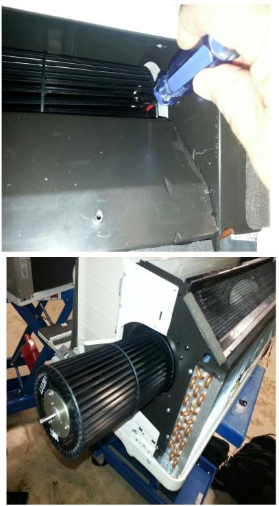
Figure 405 (Removal of Indoor Fan Blower Assembly)
