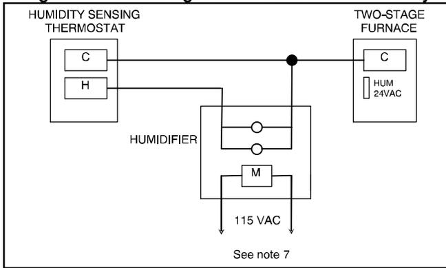
**Figure 31 – AC with Two-Stage Furnace, Humidifier, and Dehumidification**
