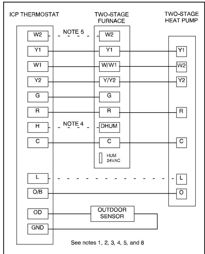
**Figure 30 – Two-Stage Furnace and Humidifier Only**
